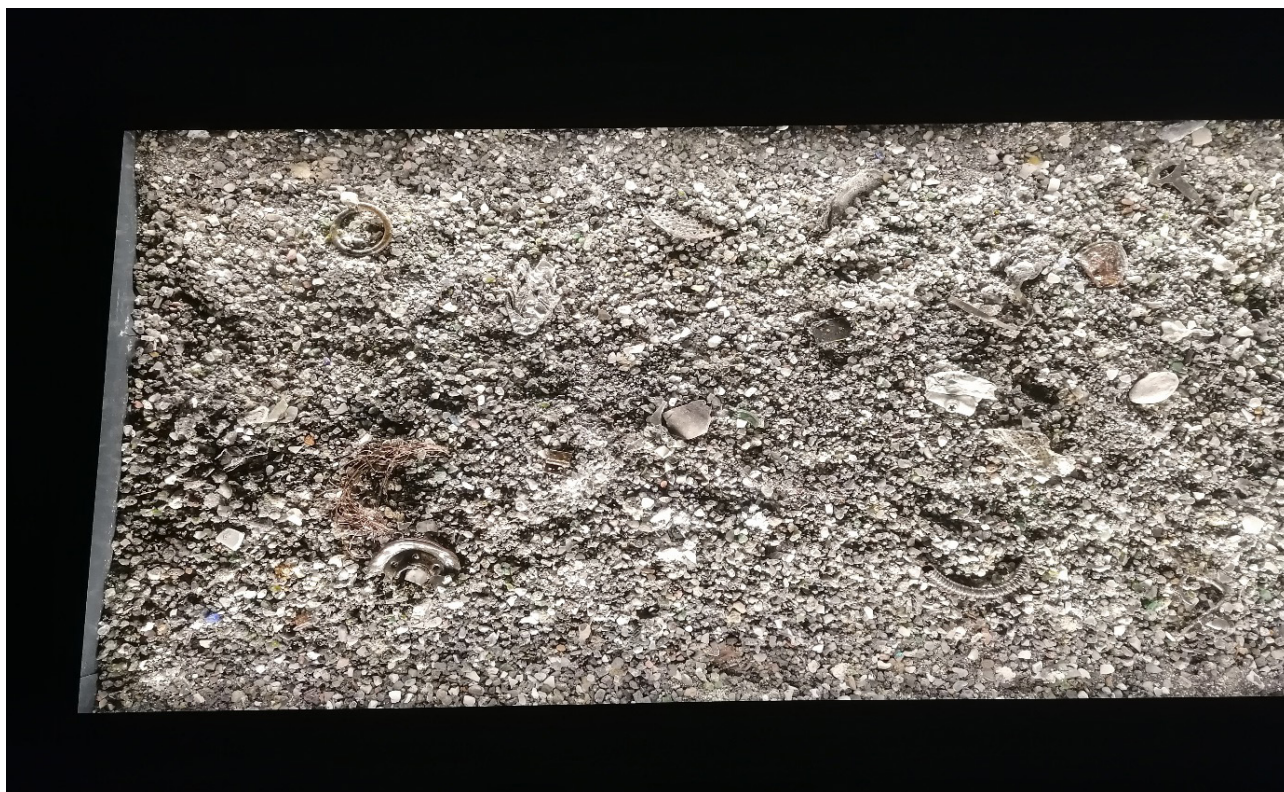
Figure 1: Solidified slag, demonstrating a granular but uniformly grey mash.
